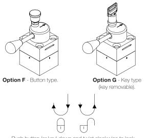
Push button (or key) down and twist clockwise to lock. Push button (or key) down and twist anti-clockwise to unlock.
