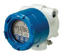
The EDD800 is a self contained digital totalizer designed to mount directly on the turbine flow meter or remotely mounted with optional hardware. The totals and flow rate units can be set to any industry standard units or be set to different units for each display. The EDD800 is easily resettable to zero out the total units displayed. The unit is available with a NEMA4 or EXP housing. Intrinsically safe,ATEX, IECEx, FM and CSA units are available.
