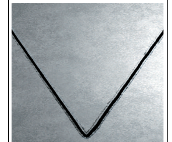
Clean cut produced by circularly polarized light.
