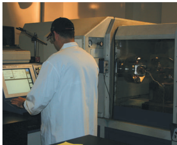
A II-VI diamond turning technician cuts spherical parts on a two-axis lathe.
