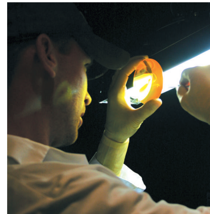
A II-VI Infrared optician evaluates a zinc selenide lens during the polishing process.
