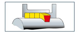
The red arrow stamp on the outside diameter of AESSTAR packing indicates the outside diameter stuffing box bore side of the packing and displays **the preferred installation orientation.** Therefore, it is recommended that the arrow mark point in the direction of the shaft rotation.
