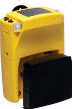
Nardalert S3 Mainframe shown with interchangeable sensor.
