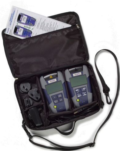
OMK-3x kit with light source, power meter, power supply, and USB cable.
