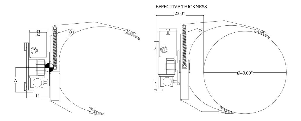
A = VERTICAL CENTER OF GRAVITY = 12 INCH UP FROM CARRIAGE BASE.
