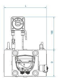
Delta DN50 G65 S1 Flow in steel and equipped with by-pass
