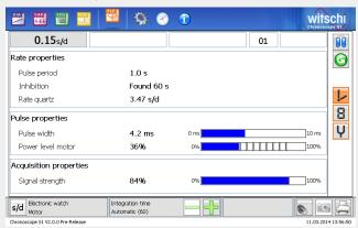
Together with the optional "Quartz Microphone" transducer for electronic watches, large numbers of electronic watches can be measured with a non-contact system. In the case of analogue quartz watches, the current rate, inhibition period, corrected rate, power level and pulse width of the motor are measured. The current rate can be specified in the case of watches with a liquid crystal display and tuning fork watches.
