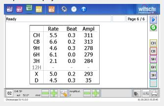
The automatic microphone Micromat S is the ideal accessory for the realisation of test sequences. When creating programs, 2 to 6 test positions can be defined including stabilisation and measuring time.
