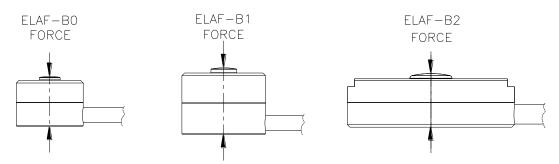
BO, B1 & B2: SPHERICAL CONTACT ON THE TOP AND FLAT SURFACE ON THE BOTTOM
