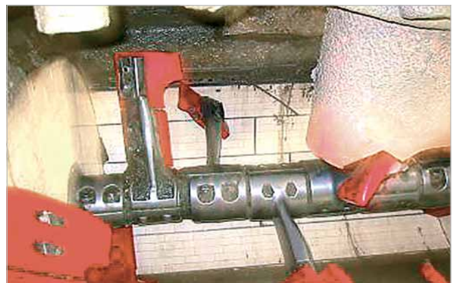
Drum mixer for concrete lined with KALOCER high alumina ceramics; mixer tools made of KALMETALL-C hard casting and/or KALEN-PU plastics
