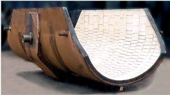
Chute for blast furnace lining in a European plant; the KALOCER lining is 50 mm thick
