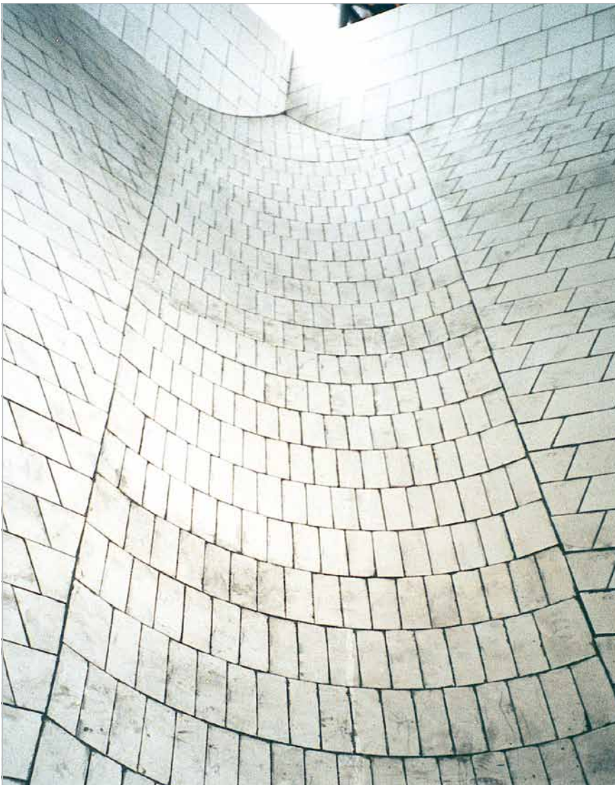
Skip collection chute with KALOCER lining installed at a European blast furnace plant; the shaped elements are up to 50 mm thick and some have been cut three-dimensionally
