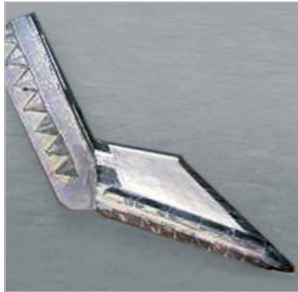
Mixer blade with KALMETALL-HM and KALOCER combined lining
