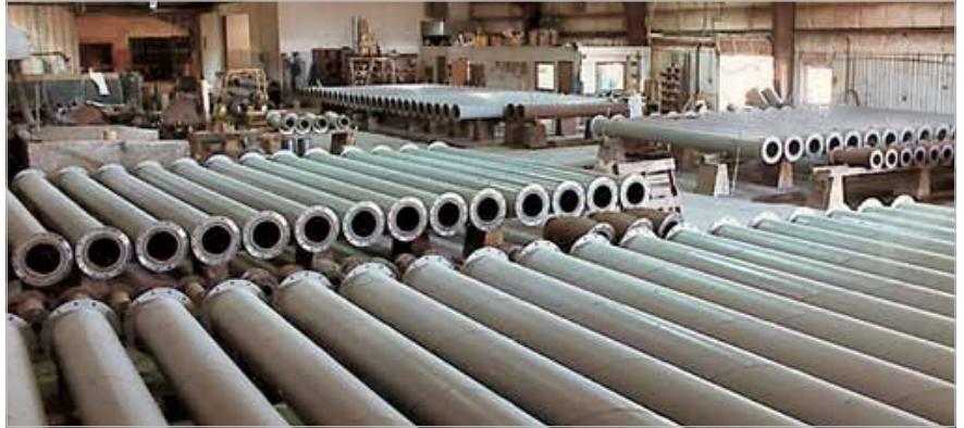
Hydraulic ash conveying pipe being manufactured at the Abresist Kalenborn Corporation plant in Indiana, USA
