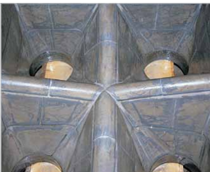
Hoppers of any shape for material discharge are fitted with ABRESIST as wear protection
