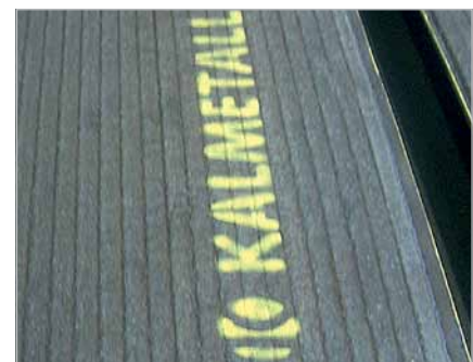
Hard overlay welded standard plates
