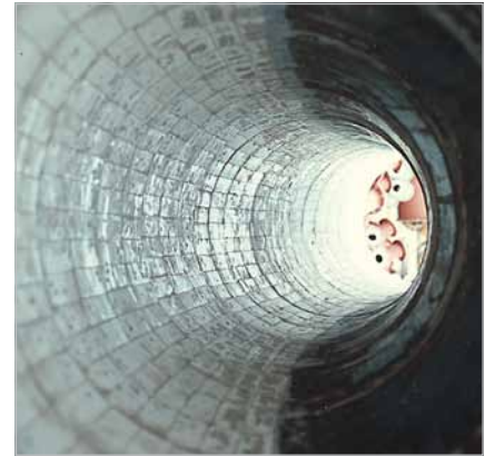
Pipe bend with ABRESIST and KALOCER combined lining
