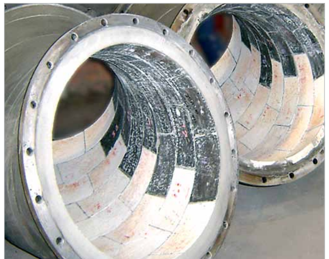
Combination of KALCOR and ABRESIST in a pulverized coal pipe in Europe
