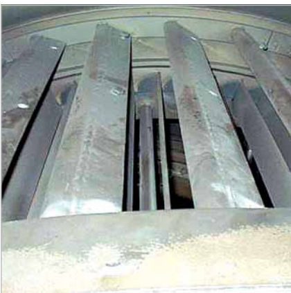
Guide vanes of a separator made of KALSICA-A operated within a coal pulverizer
