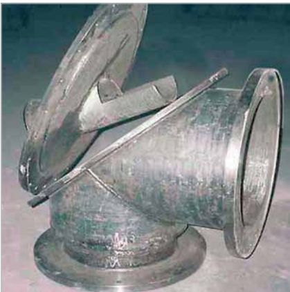
Pulverized coal burner lined with KALMETALL-W 145
