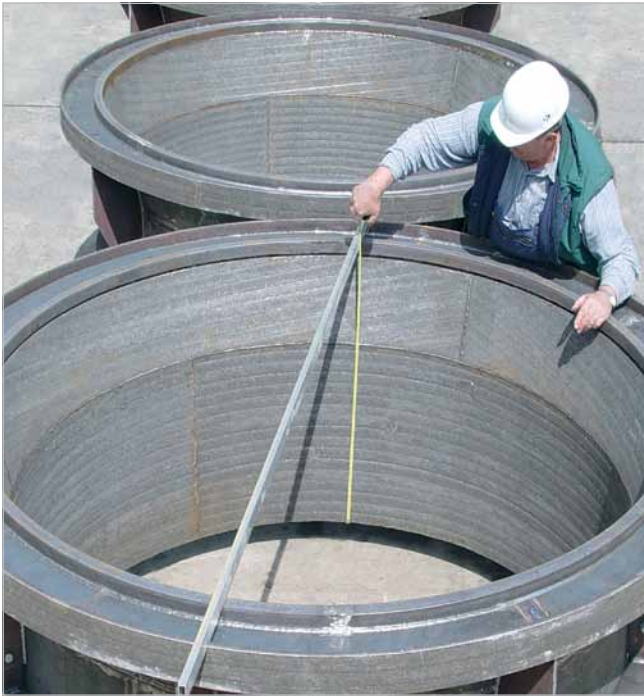
Separating cones of cement classifiers made of KALMETALL-W 100 as self-supporting structures
