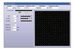
The MSQ-PC also provides users with access to more QAM measurements, such as the constellation diagram of the QAM signal, which is not visible on the MSQ-800 meter itself.
