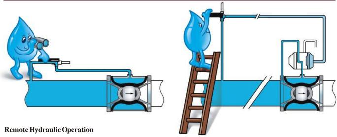
Operation of the **Inbal** Valve is also available by a release valve, installed remotely on a control panel, located in an accessible spot.
