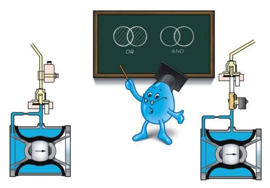
Non-interlock pneu-electric release control. The **Inbal** Valve will open either upon the operation of the electric release or a drop of pressure in the dry pilot line.
