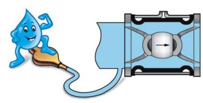
When no pressure acts on the valve, the resilient heavy duty sleeve holds the **Inbal** valve closed.
