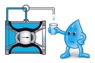
The **Inbal** Valve closes tightly when the pressure port is interconnected with the common port. The vent port is isolated.
