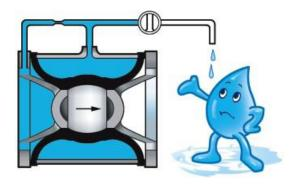
The **Inbal** Valve closes tightly when the flow rate introduced to the control chamber is greater than the released flow rate. Obviously, if there is no outgoing flow rate, then the closing speed is faster.
