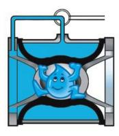
The **Inbal** Valve closes when inlet pressure is applied to the control chamber. The equilibrium in pressures and forces acting on the sleeve maintains the valve in a closed position.
