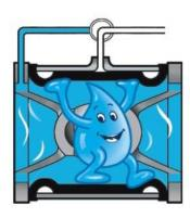
The **Inbal** Valve opens wide when the operating pressure is relieved from the control chamber. A minimum line pressure is required to hold the **Inbal** Valve in a fully open position. The flow through the valve is streamlined with low pressure loss.
