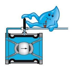
Operation of the ½" release valve is all that is needed to open the **Inbal** Valve. The operator can move on to other tasks while the **Inbal** Valve completes the opening process, to a fully open position, fairly quickly but with no surges.
