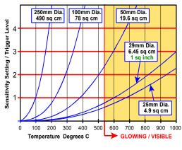
The chart (left) indicates the correlation between the temperature and size of 'hot spot' anomalies for a typical installation to produce one or more detector channel activations at various trigger level settings
