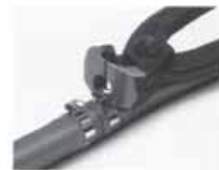
use of side jaw pincer held parallel to hose
